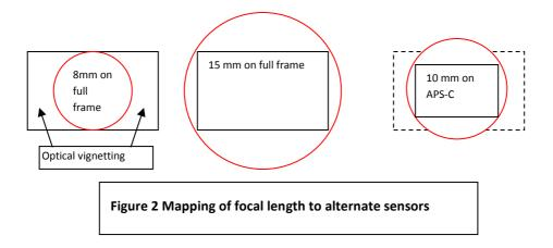
The Canon APS-C sensor provides a maximum resolution of  $5472 \times 3648$  pixels. The standard full frame (35.9 x 24 mm) provides resolutions up to  $6240 \times 4160$  pixels.
